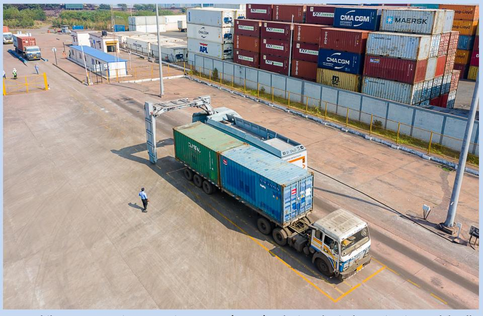
Mobile X-Ray Container Scanning System (MXCS) reducing physical examination and dwell time of containers at VCTPL.
